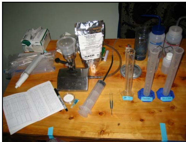
Figure 3-6: Membrane Filtration Equipment
