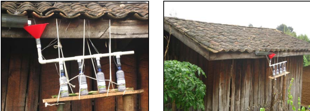
Figure 3-12: PT array on old clay-tile roof
