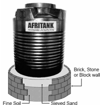
Figure A-14: Typical AFRITANK plastic water collection tank with foundation (Kentainers undated)
