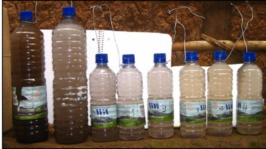
Figure 3-37: Turbidity at HS location, storm S4 (Bottles A through H are from left to right)
